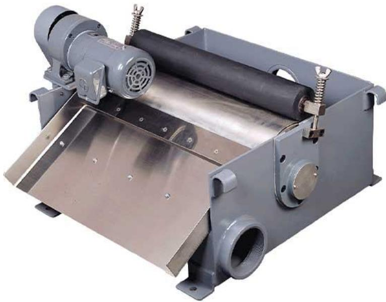
A **Magnetic Separator** is a device used to remove ferrous and non-ferrous contaminants from a variety of materials. It works by utilizing powerful magnets to attract and hold onto the magnetic particles, while allowing the non-magnetic particles to pass through. *Magnetic Separators* are widely used in industries such as mining, food processing, pharmaceuticals, and recycling, among others.
